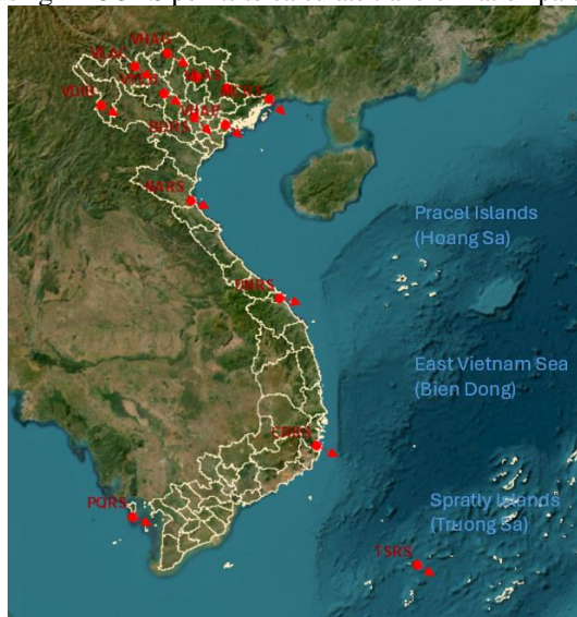
Figure 4.2: Direction of displacement of the 14 measurement points Table 4.1: Transformation parameters calculated using 14 CORS points
